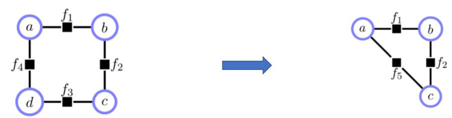
$p(a, b, c, d) = f_1(a, b) f_2(b, c) f_3(c, d) f_4(a, d)$
