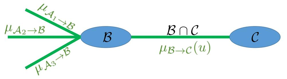
$$\mu_{\mathcal{B}\to\mathcal{C}}(u) = \sum_{v\in\mathcal{B}\setminus\mathcal{C}}\psi_{\mathcal{B}}(u\cup v)\prod_{\substack{(\mathcal{A},\mathcal{B})\in\mathcal{E}\\\mathcal{A}\neq\mathcal{C}}}\mu_{\mathcal{A}\to\mathcal{B}}(u_{A}\cup v_{A})$$
